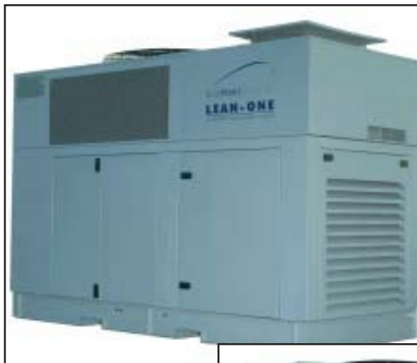
BluePoint Energy's 260 kW Lean-One CHP module is equipped with a 325 hp Deutz gaseous-fueled engine incorporating EGR and a stoichiometric catalyst package.
